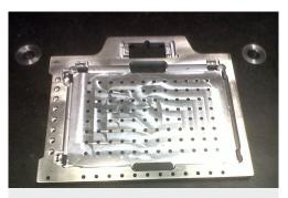
Finished component of a blood analysis machine manufactured by Talleres Cridi.
